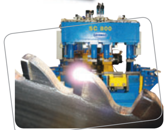
Rail Carbide Cutting Machine, SC 800 type
